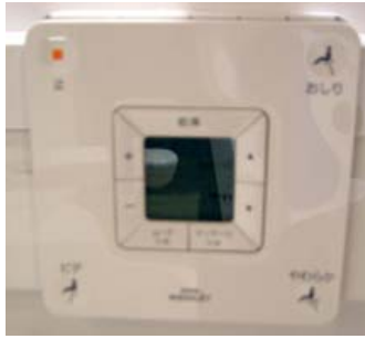
Fig. 6. More, inclusive design of bidet toilet control by Sekisui House, Japan
