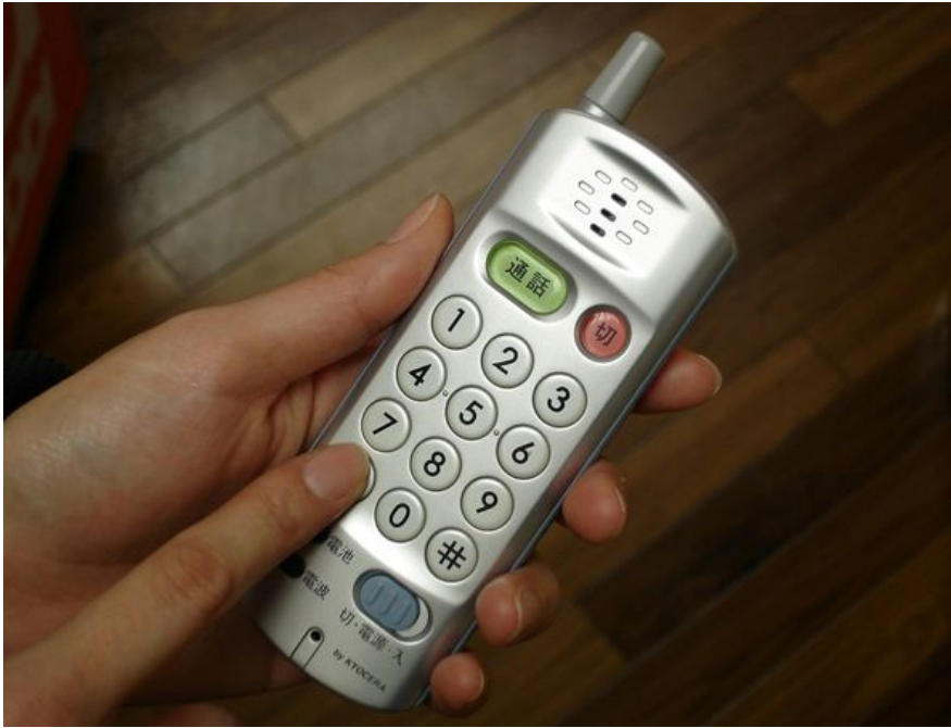
Fig. 1. Kyocera’s TU-KA S mobile displaying a simplified interface with enlarged buttons and characters
