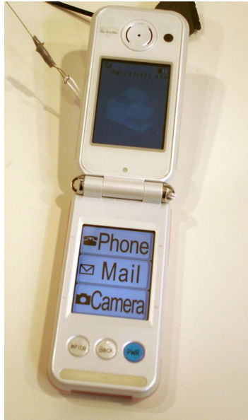
Fig. 3. Mitsubishi's D800iDS twin-screen prototype (as at October 2006) now available on the market. The lower screen is a touch-screen and the interface can be customized to the user's preferences.
