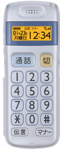
Fig. 2. NTT DoCoMo’s Raku-Raku mobile by Mitsubishi, 2006, showing the ‘talk’ (blue) and ‘end’ (orange) buttons and small screen. A small internal drawer extends from the bottom end of the mobile on which the customer can write phone numbers.
