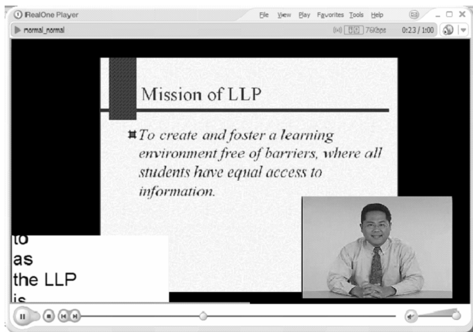
Fig. 3. The figure shows a sample of ill defined layout, where presentation image is surrounded by excessive empty space. Video and caption overlap with the presentation image. The caption is being cut off by the window boundary.
